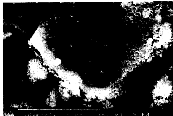
Fig.8: Surface of a spherical void (1.2mm \varnothing ) in dolomite filled epoxy after 2400h of exposure to discharges (SEM picture).
