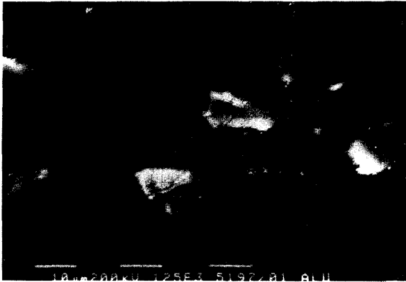
Fig.3: Surface of alumina filled epoxy before discharges.
