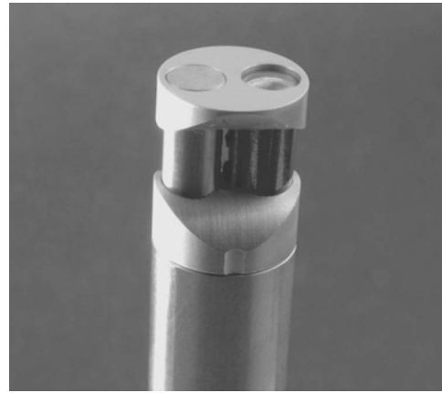
FIG. 2. The Microflow \frac{1}{2} -in. sound intensity probe.
