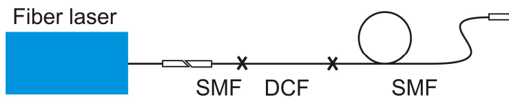
Fig. 1. Fiber link design. The output of the fiber laser is butt-coupled to the fiber link using FC/APC connectors. The crosses show where SMF and DCF fiber sections are spliced together.
