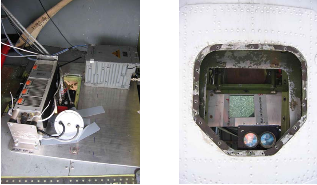
Fig. 10. Left: Riegl laser scanner with attached heating pads (left) and EGI instrument (back right). Right: Aircraft hole photographed from below, with scanner mirror and below the lenses of single beam laser altimeter (backup instrument). The web camera was mounted just left of the two lenses.
