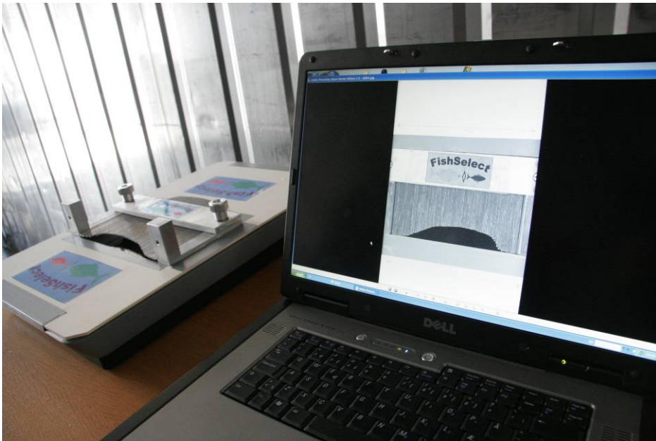
Fig. 4. Experimental setup of the process of scanning the MorphoMeter with the outline of the cross section and acquiring the data in a laptop computer.
