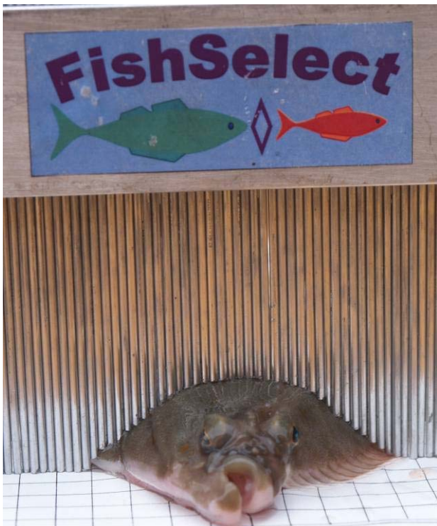
Fig. 2. Plaice in MorphoMeter. CS1 is being measured.
