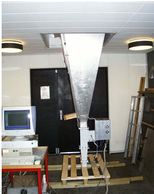
Figure 4. Setup of the EMIRAD L-band radiometer inside the roof-top shelter. The antenna is zenith looking, and it is located behind a small window for long-term measurement.
