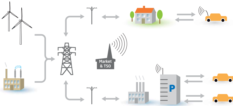
Fig. 12.5. Electric vehicles with vehicle-to-grid functionality can dynamically communicate with and exchange power with the electric power system and thereby ensure real-time balancing of the fluctuating wind power. TSO: transmission system operator.
