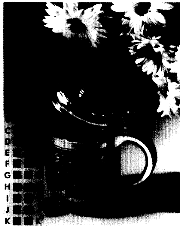
Fig. 11. Reconstruction from scanned test image shown on Fig. 10 using the (4,2) Wiener filter.
