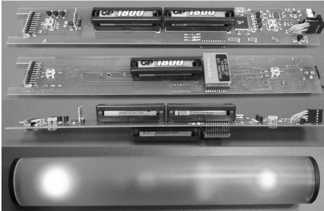
Fig. 5. PCB seen from the top, the bottom, the side, and an assembled RP.
