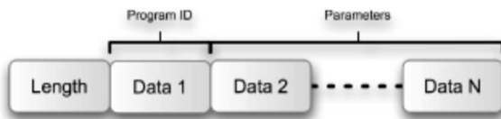
Fig. 13. Transmission package structure.
