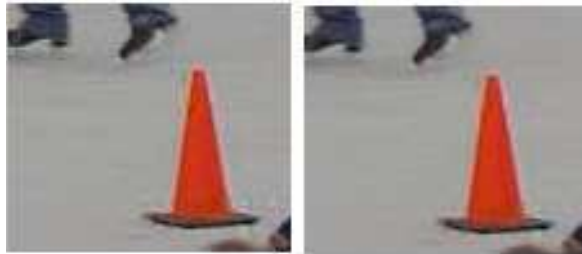
Figure 4: MPEG2 Decoding without (left) and with deringing (right). Part of frame 18 of ICE.
