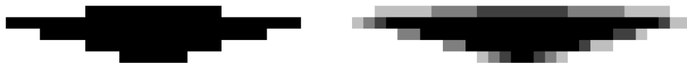
Figure 26: The difference between no anti-aliasing on the left and anti-aliasing with 16 samples per pixel on the right.
