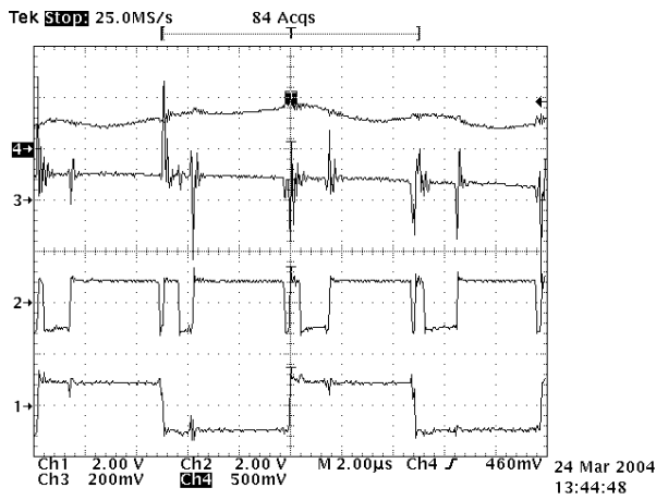
Fig. 10. Detailed SICAM operation: 1) HF-link voltage (100V/div), 2) bridge voltage (100V/div), 3) voltage reference (2V/div), 4) output voltage (5V/div) with 10 kHz reference
