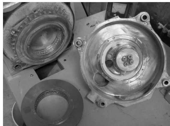
Figure 1: Disassembled California Pellet mill (25 kg/h) showing the ring matrix in the upper left corner. The roller is shown to the right.
