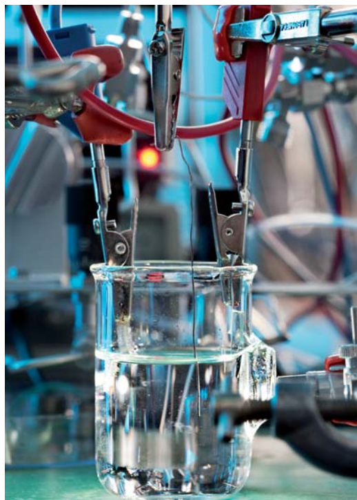
Fig. 2.7. The photocatalytic cell combines harvesting of light into electron-hole pairs and using them to split water into oxygen and hydrogen directly. This requires carefully designed materials to use a large part of the solar spectrum and a good catalyst for the electrochemical process where hydrogen and oxygen are evolved.
