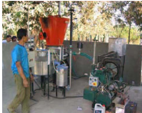
Figure 4.5 Biomass gasifier in Anlong Tamey. Source: JICA study of rural electrification by Renewable energy in Cambodia
