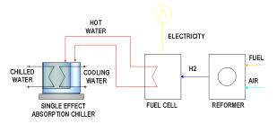
Figure 6. Schematic diagram of the FC+SE trigeneration system
