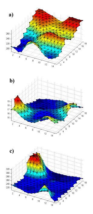
Figure 4: The component planes of different emission components  $[mg/Nm^3]$ , a) NO<sub>x</sub>, b) CO and c) SO<sub>2</sub>, on 18\*14 SOM grids after modeling the process state of **high steam flow**.
