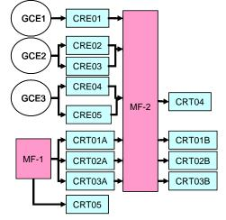
Figure 13: A subnetwork of South East Kuwait Crude oil pipeline network.
