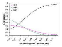
Figure 9: Composition of the bubble point gas phase of a 10wt% ammonia solvent with a temperature of 110°C as a function of the CO<sub>2</sub> loading
