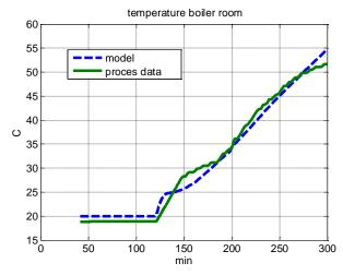
Figure 7: Temperature in boiler room
