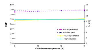
Figure 10: COP and cooling capacity (Qc) with MGT output of 20 kW and air temperature at 28  $^{\circ}$ C inside the environmental chamber.
