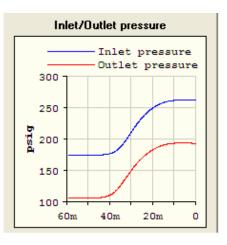
Figure 7: Pressure at the inlet and outlet of pipeline CRN121 after implemented remedies.
