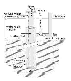
Figure 2: Dual-Gradient Drilling flow schematic
