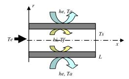
Figure 2.Physical model for the condenser, evaporator, the absorber and the collector.
