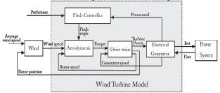
Figure 5: Block diagram of Wind Turbine system
