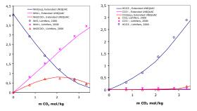
Figure 4: Speciation calculations at 80°C for a molality of ammonia of 4.1mol/kg
