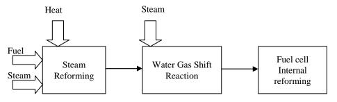
Figure 3 Fuel reforming process
