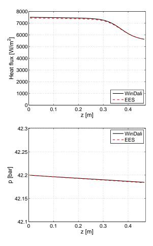
Figure 4: Comparison of the local heat flux and pressure in the channel for refrigerant  $CO_2$  with uniform distribution of the airflow.
