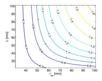
Figure 4: Contours of the mean flux density as a function of external radius and length. Each contour is labeled by its mean flux density. The maximum flux density is obtained by maximizing both  $r_{ex}$  and *L*.
