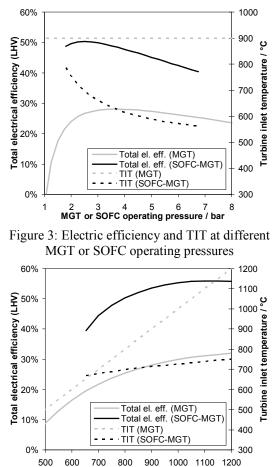
TIT or SOFC operating temperature / °C Figure 4: Electric efficiency and TIT at different
