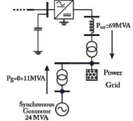
Figure 16: Study case for assessing the frequency control function
