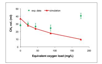
Figure 5: Experimentally determined (average±SD) and simulation predicted ultimate methane generation vs. oxygen load
