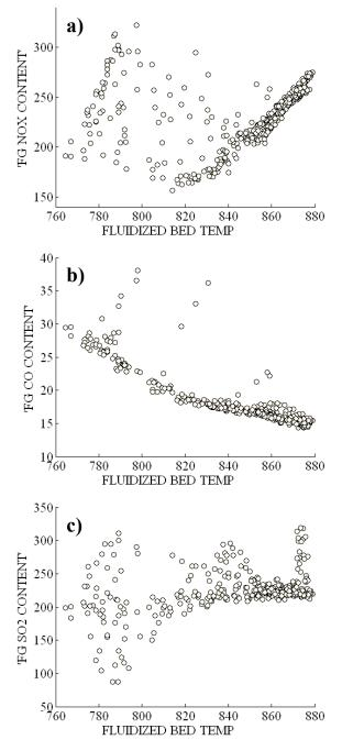
Figure 2: Emission models after creating a 24\*16 SOM. a) NO<sub>x</sub>, b) CO and c) SO<sub>2</sub> content [mg/Nm<sup>3</sup>] of flue gas (FG) as a function of the bed temperature [°C] by using the reference vectors of SOM neurons.
