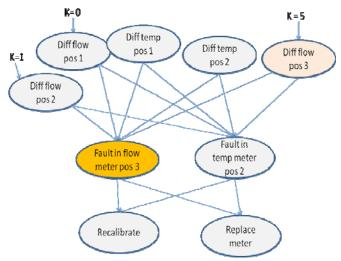
**Figure 4.** Decision support on possible faults from the previous example
