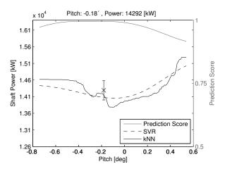
Figure 8: An example of how a prediction score can be displayed along with predicted values. The score indicates reliable predictions of values from -0.4 to -0.05.
