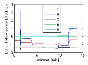
Figure 3 Main effects on bottomhole pressure
