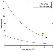
Figure 8. Distribution of the wall and the fluid temperatures for the evaporator.
