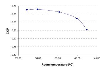
Figure 4: COP of the absorption chiller as a function of ambient temperature for an electrical output power of 20 kW, a chiller temperature of 8°C and a thermal oil flow rate of 2400 l/h
