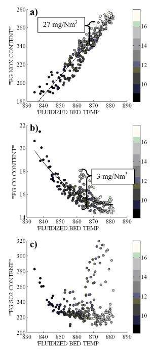
Figure 5: Emission models of the process state of high steam flow. a)  $NO_x$ , b) CO and c)  $SO_2$  content [mg/Nm<sup>3</sup>] of flue gas (FG) as a function of the bed temperature [°C] by using the reference vectors of SOM neurons. Color scale indicates the deviation of the bed temperature [°C].
