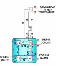
Figure 2. Schematic diagram of a DE absorption chiller
