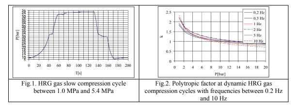
Similar stability of the HRG gas has been observed also during dynamic compression/decompression tests at frequencies between 0.2÷10 Hz and maximal pressure until 1.8 MPa [5].
