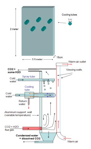
Figure 2 Proposed geometry for condensation study
