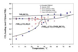
Figure 2: Phase diagram for the ammoniacarbon dioxide-water system from -6 to 90°C
