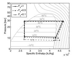
Figure 5:  $\log p$ -h diagram at different  $F_x$  (case 1)
