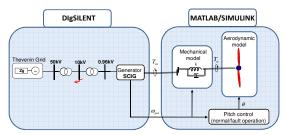
Figure 3: Splitting the task of simulation between DIgSILENT and MATLAB/SIMULINK.
