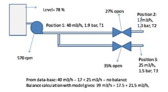
Figure 2 A simple example of a system to illustrate the procedure
