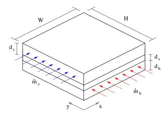
Figure 1: A simple illustration of a cross flow heat exchanger
