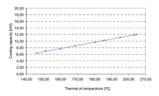
Figure 7: Cooling capacity of the absorption chiller versus thermal oil temperature for an ambient temperature of 35°C and a chilled water temperature of 8°C
