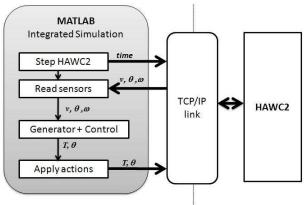
Figure 4: Integrated simulation simplified flow diagram
