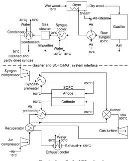
Figure 1: Flow sheet of the hybrid systems
