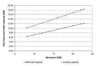
Figure 6: Heat input and capacity of the absorption chiller versus MGT electrical power output for an environmental chamber temperature between 25 and 35°C and a chilled water temperature of 8°C
