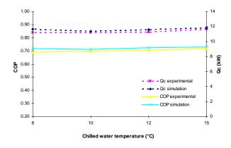
Figure 9: COP and cooling capacity (Qc) with an MGT output of 18 kW and an ambient temperature of 27  $^{\circ}$ C inside the environmental chamber.
