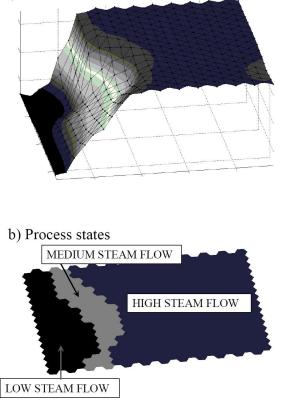
Figure 3: a) The behavior of the main steam flow on a 24\*16 SOM, and b) Clustered SOM (k = 3), which shows the separation of process states into three categories.
