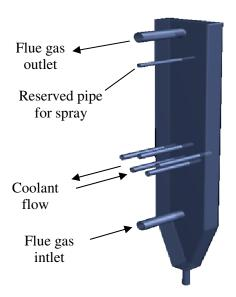
Figure 3 First implemented model for condenser
