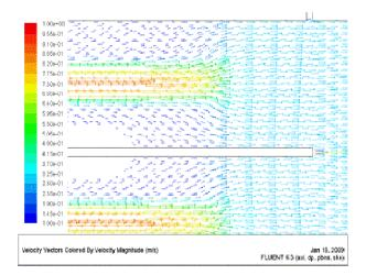
Figure 7: Contours of distribution of the Velocity vectors around the outlet of the lower channel
