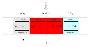
Figure 2: An assumed isothermal hot junction of the single-couple TEG.
