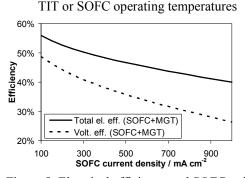
Figure 5: Electrical efficiency and SOFC voltage efficiency as a function of SOFC current density
