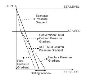
Figure 1: Hydrostatic pressure profile for dual gradient and conventional drilling
