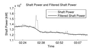
Figure 4: The shaft power series and a filtered shaft power series where the outlier has been discarded.
