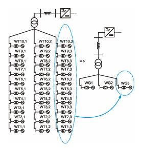
Figure 6: Multi-machine equivalent
