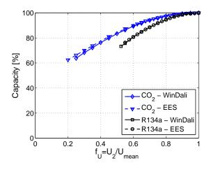
Figure 7: Comparison of the reduction of cooling capacity due to maldistribution of the airflow for R134a and  $CO_2$  using both EES and WinDali.
