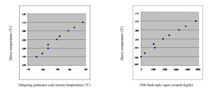
Figure 3: The effect of increasing slurry temperature on the generation of vapor by V06 and the preheater cold stream temperature
