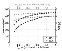
Figure 8: Evaporator UA-value and COP vs.  $F_{air}$  (case 3 and 4)
