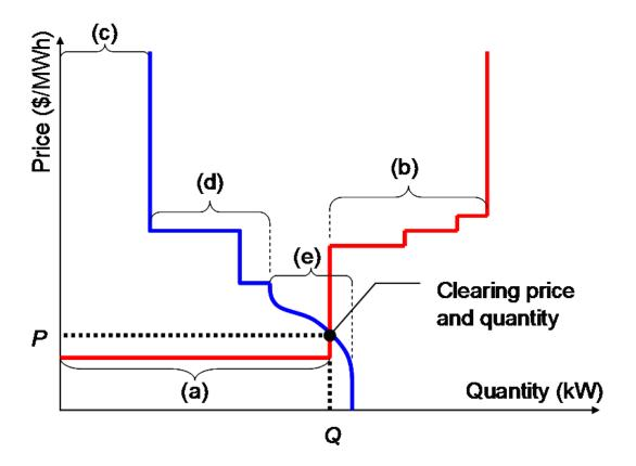
Figure 2 - Double auction for distribution feeder capacity
