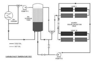
Figure 1: Layout of the Acurex solar collector field.
