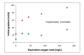
Figure 2: Initial gas generation rates under different oxygen loading conditions
