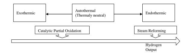
Figure 5 Hydrogen output as function of operating conditions
