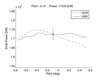
Figure 6: An example of a poor shaft power prediction for pitch values far from zero. The vertical segment through the known data point, marked with X, shows the RMS error of 290.
