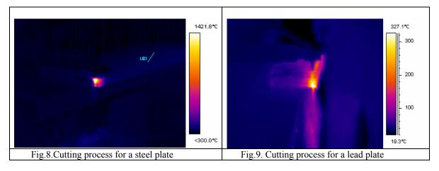
The temperature distributions observed in cutting process showed a consistent energy density in the process core (fig. 8, 9).
