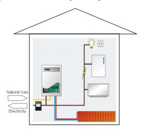
Figure 1 Household micro CHP system based on SOFC
