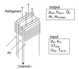
Figure 1: Sketch of two channels in parallel with input and output parameters to the model.
