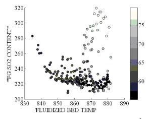
Figure 6: Flue gas (FG) SO<sub>2</sub> content [mg/Nm<sup>3</sup>] as a function of the bed temperature [°C] by using the reference vectors of SOM neurons in the process state of high steam flow. Color scale indicates the deviation of the furnace middle level temperature [°C].
