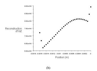
Figure 7: Temperature gradient distribution in an xy plane corner line along z direction. (a) ANSYS. (b) FLUENT.
