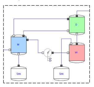
Figure 4: Dilution tank (D), Mixing tank (M) and Electrowinning tank (W)
