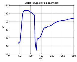
Figure 6: Temperature of water into economizer
