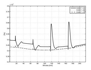
Figure 10: Estimated friction parameter in annulus
