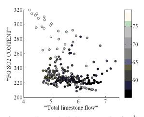
Figure 7: Flue gas (FG) SO<sub>2</sub> content [mg/Nm<sup>3</sup>] as a function of the limestone flow [kg/s] by using the reference vectors of SOM neurons in the process state of high steam flow. Color scale indicates the deviation of the furnace middle level temperature [°C].
