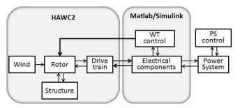
Figure 1: Wind power integrated design platform: HAWC2 - Matlab
