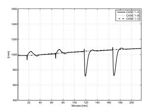
Figure 9: Estimated flow through bit
