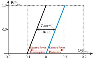
Figure 1: Reactive power control requirements
