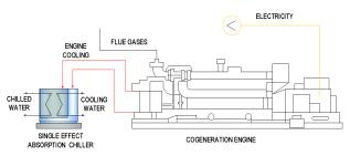
Figure 5. Schematic diagram of the ICE+SE trigeneration system
