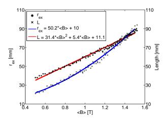
Figure 6: The optimal  $r_{ex}$  and *L* as functions of the mean flux density. Polynomia have been fitted to the data to ease interpolation. Building a Halbach cylinder with an internal radius of 21 mm with dimensions different from the dimensions given here means that more magnetic material is used than need be, if one does not care about the volume of the bore.
