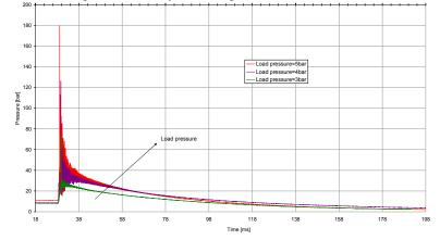
Fig.4. Auto-ignition moment of the HRG gas combustion heated in a bomb
