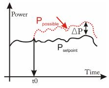
Figure 12: Delta production constraint
