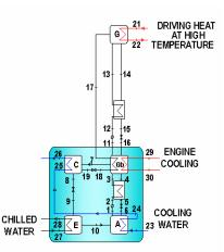
Figure 3. Schematic diagram of a SE/DE absorption chiller
