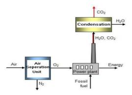
Figure 1 schematically representation of oxy-fuel process
