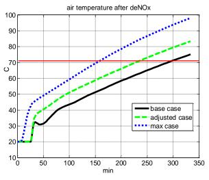
Figure 9: Air temperature after deNOx
