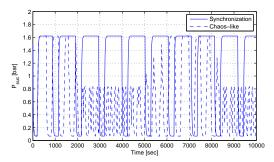
Figure 5: The suction pressure  $P_{suc}$  in the situations of (a) synchronization ( $\underline{T_{air,2}} = 0$ ) and (b) chaos-like ( $T_{air,2} = 0.3$ ).
