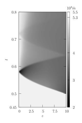
Figure 5: The space-time dependence of  $\dot{m}$  as the outlet volume flow  $\dot{V}$  is reduced by a factor of two at t = 0.5 s. A pressure wave is seen to rapidly shuttle back and forth a few times. Units refer to Table 1.
