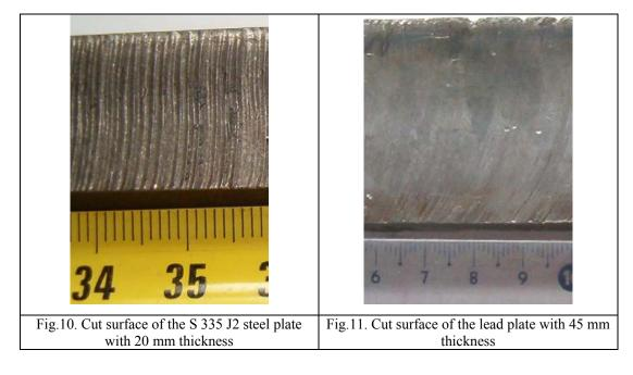
Some interesting aspects can be mentioned here concerning the fig. 10 and 11: stability of the cutting process due to the flame uniformity and the almost non-chamfered edge the cut surface which was much closed to the first stage of the HRG flame in the spite of the magnitude of the plate thickness. In the fig.10 it is about high yield
