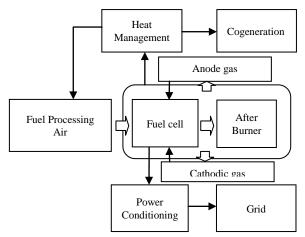
Figure 2 Micro CHP system configuration
