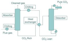
**Figure 1: Flow sheet of the process**
