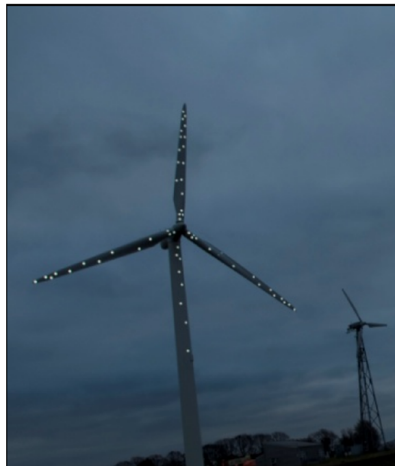
Figure 5: View of the fully targeted rotor and tower during flash testing. It can be seen that the high power flash has successfully illuminated all of the retro-reflective targets.
