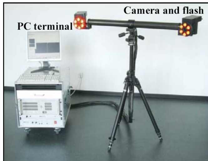
Figure 3: Standard PONTOS sensor comprising heavy-duty carbon fiber camera support, stereo pair of 500 fps cameras, synchronized ring flashes, and computer for data acquisition control, image processing, and comprehensive analysis, reporting and data export software features.
