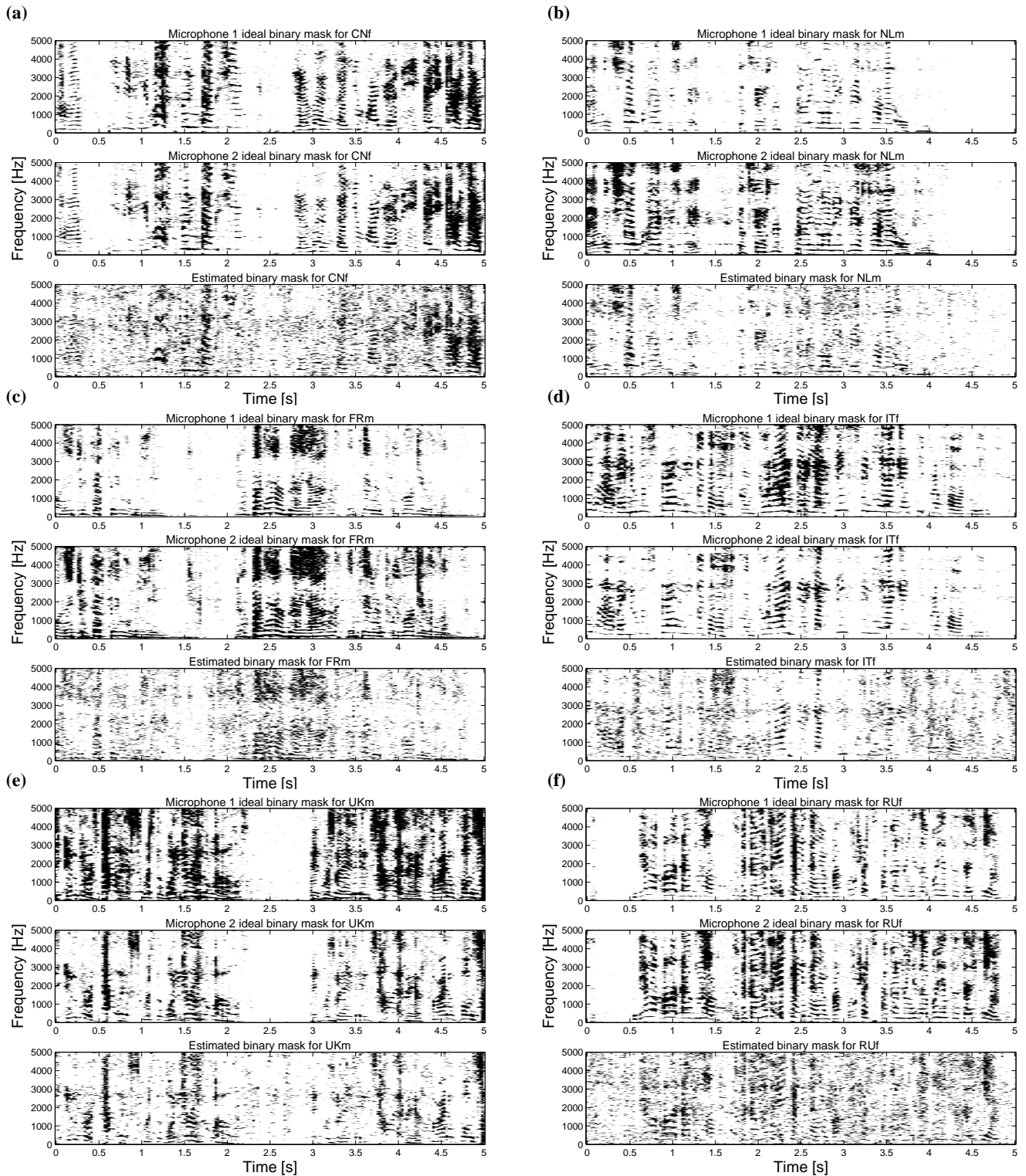
Fig. 5. For a mixture of 6 mixed speech signals, binary masks have been estimated for each of the 6 speech signals. The black areas correspond to the mask value '1' and the white areas correspond to the mask value '0'. The results are shown together with the calculated ideal binary masks of each of the two microphone signals. The signals (a)–(f) appear in the order which they were extracted from the mixture. The first three signals (a)–(c) were extracted after two iterations, the next two signals (d), (e) were extracted after three iterations. The last signal (f) was extracted from the remaining mask as described in section 3.2.
