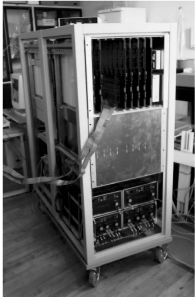
Fig. 6. The RASMUS scanner seen from the front with the receivers on the top, the transmitters in the middle, and the power supplies in the bottom. The analog front-end and transducer connection along with a control PC is placed in the other rack cabinet.
