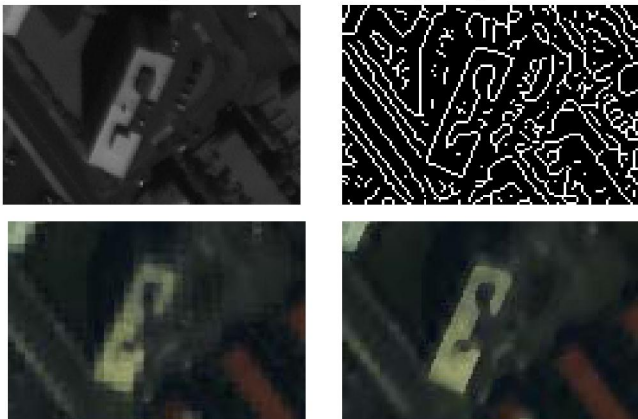
Fig. 1. A sample of the images: top left: Pan-chromatic image. top right: Extracted lines. bottom left: Initial estimates via (4) bottom right: Fused image via (11). The colors in the bottom row correspond to the red green and blue channel respectively.
