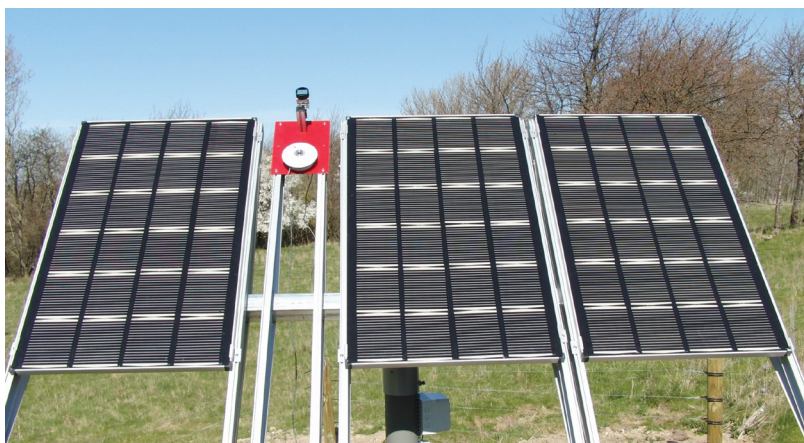
In April 2009 Risø demonstrated the world first grid connected polymer solar cells.
