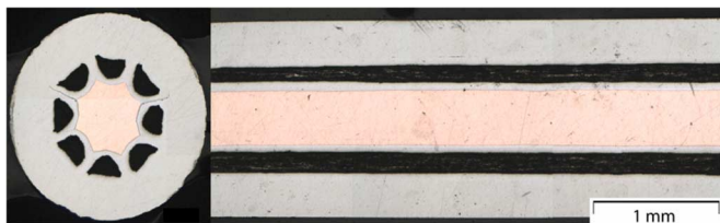
Fig. 4. Specimen "i", 8-filament wire with copper core using in-situ powder, annealed once.
