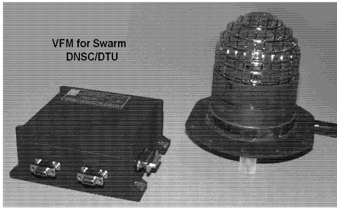
Fig. 10. New generation of the high precise space vector magnetometers with compact-spherical-coil designed at DNSC and involved in ESA Proba2 and ESA SWARM missions
