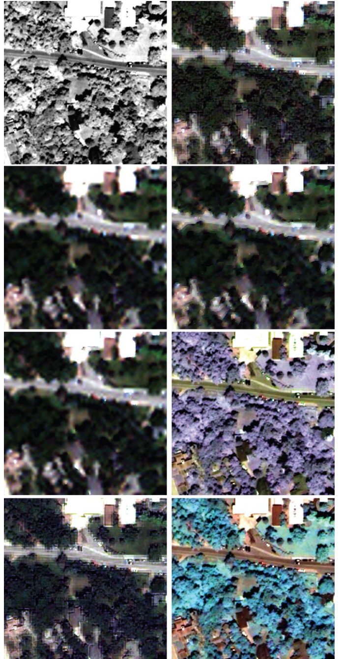
Fig. 6. Results of the image fusion strategies. A sample of the resulting images of the QuickBird data set. (Top left) Input panchromatic image. (Top right) No smoothing. (Row 2 left) Uniform weights. (Row 2 right) Edge-induced weighting. (Row 3 left) Gradient-induced weighting. (Row 3 right) IHS method. (Bottom left) Mean-corrected IHS method. (Bottom right) Brovey method. The images have been stretched for better visualization.
