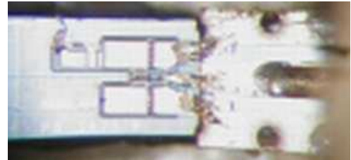
Fig. 7 Micro-photograph of the packaging of the original photodetector module as well as a PD chip.
