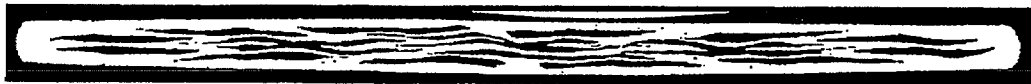
Fig. 1: Cross sectional view of a superconducting BSCCO-2223 tape with 19 filaments. The dimensions are 3.5×0.2 mm. The dark area inside the bright grey area (silver metal matrix) is the actual superconducting material carrying the current.
