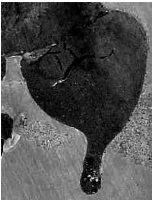
**Figure 8.** Basalt droplet captured in the quenched cupola. (The total width of the picture is 70mm.)
