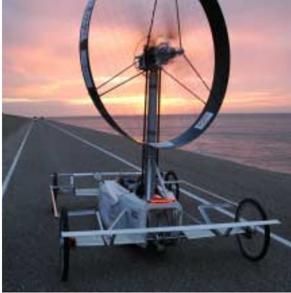
Figure 2: Example of a wind car: the WindTurbineRacer [4] racing along the dike, against the wind at the 2008 Aeolus race in Den Helder, the Netherlands.
