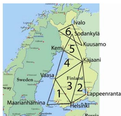
Figure 5: The triangles used in the calculations of geostrophic wind speed. Triangle 1 used pressure observations, reduced to sea surface level, from Helsinki, Mariehamn and Vaasa.
