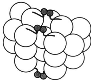
FIG. 1. The geometry of an H_2 molecule along the minimum energy path approaching an Al(110) surface. A molecule approaches the surface in each of the (1 \times 2) unit cells and on each side of the five-layer slab used in the calculation, but the interaction between the molecules is small and does not affect the results.
