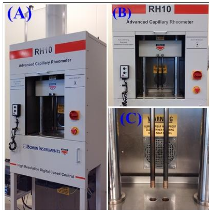
Figure 3.17 Rosand RH10 (A), front view (B) and rods and reservoirs (C)
