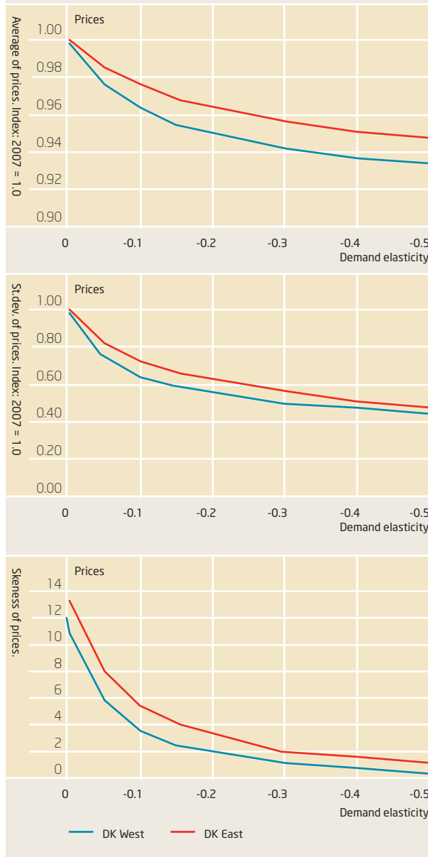
Figure 27 Demand price elasticity and changes in the average, standard deviation and skewness coefficient for the distribution of hourly prices, 2007.
