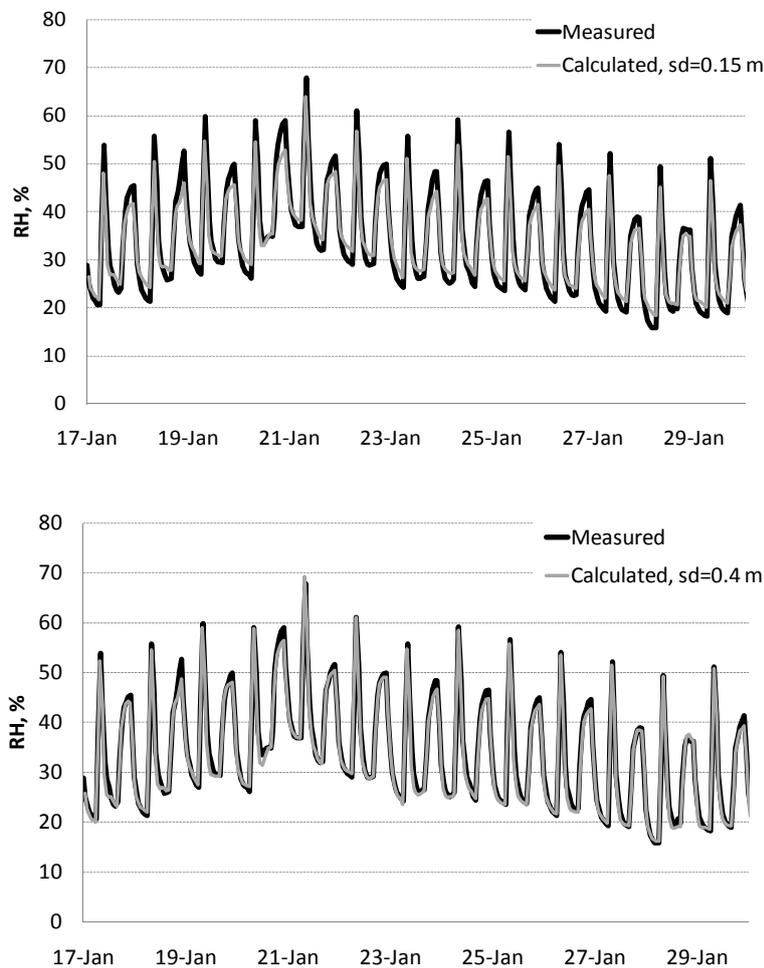
FIG. 4. Relative humidity in the reference room. Black line shows the measured values, the grey line shows the calculated values with  $s_d=0.15$  in the upper figure and  $0.4$  m in the lower figure. The ventilation flow rate is  $0.63$  1/h in all cases.
