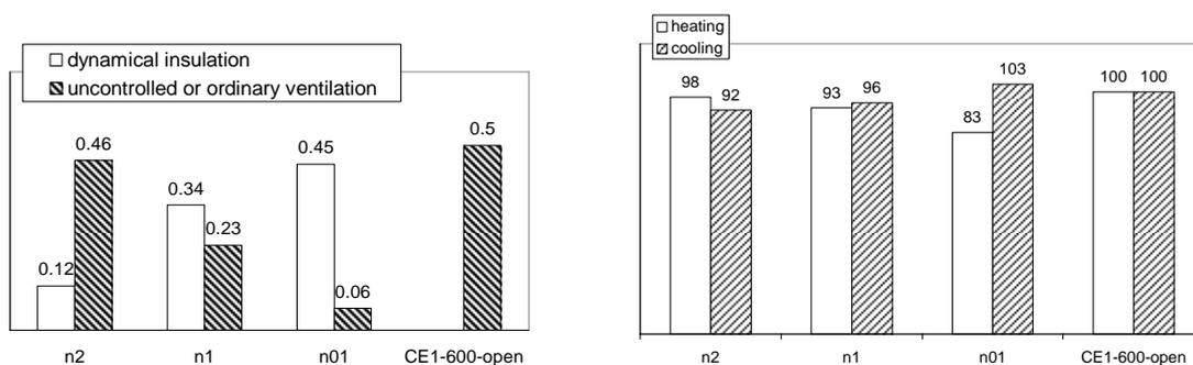
FIG 5. Left: Airflow rates (annual averages) through the dynamical insulation in the roof and thorough the air leakages in the building envelope, in relation to the overall airtightness of the building envelope. n2 stands 2 1/h at 50 Pa pressure difference, etc. The case CE1-600-open refers to the calculation exercise CE 1, with a lightweight and vapour-open construction. Right: Annual energy consumption for heating and cooling in kWh, for the cases from the figure to the left.
