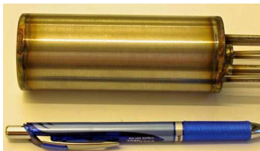
Fig. 5 Ammonia cracker prototype for generating 6.75 nL/min H 2
