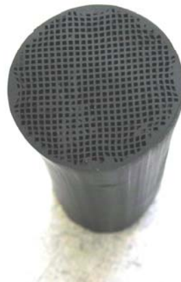
Figure 7: A piece of an extruded structure. The structure contains a regular array of square holes separated by thin walls of the magnetic ceramic material LCSM material.
