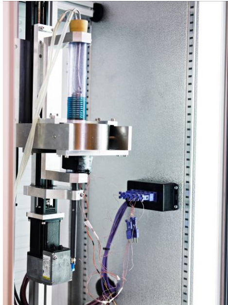
Figure 4: The test device at Risø DTU, showing the tube containing the heat transfer fluid within a cylindrical magnet.
