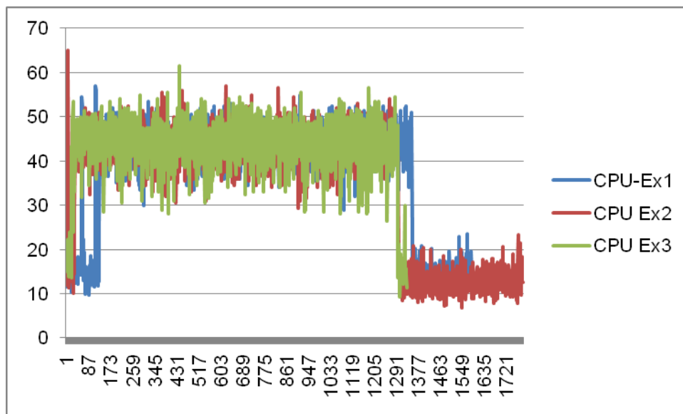
Figure 3-17: Analysis of CPU Utilisation against ICMP Flood
