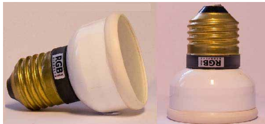
Fig. 3. The LED Bulb prototype used in the experiments, it was created by RGB Lamps.
