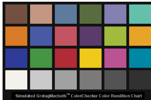
Fig. 5. A simulated "ColorChecker" chart from Gretagmacbeth, typically used when comparing different illumination sources with each other. [22]
