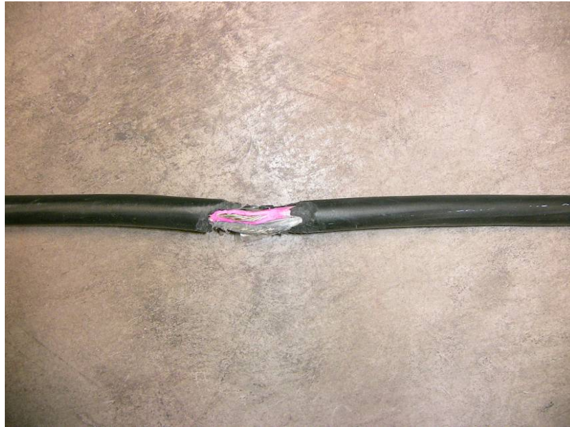
Figure 3 TXM2 gouge of 2 wires (dry)
