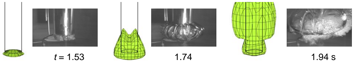
Figure 5. Formation of gas bubble at the vent outlet in the pressure suppression pool. Comparison of FSI calculation to experimental results obtained at PPOOLEX facility.
