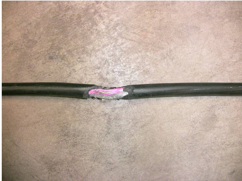
Figure 3 TXM2 gouge of 2 wires (dry)
