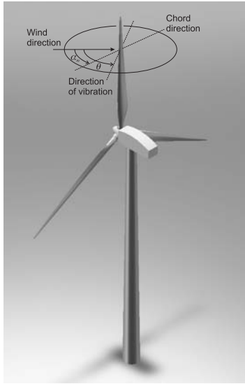
Figure 104. Stall-induced blade vibrations of wind turbine at standstill may occur when the wind direction relative to the airfoil chord and the direction of vibration for a blade mode is critical.
