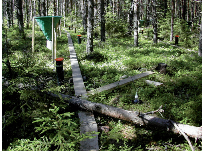
Figure 4. Samplers on a FIP plot. Litterfall samplers (green funnel), stand throughfall samplers (orange) and a bottle to collect soil water through lysimeters are shown.
