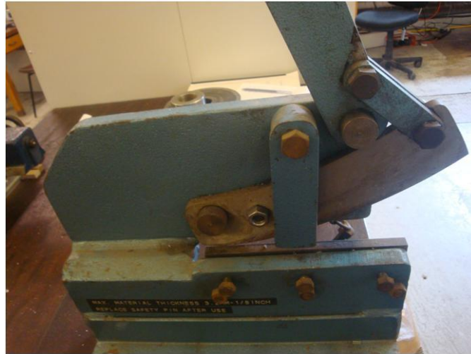
Figure 4.41: Keeton cutter machine used to dimension the length of the drawn samples
