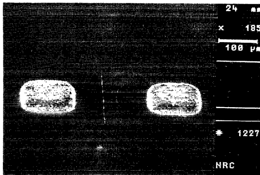
FIG. 6. The 140\ \mu\text{m} \times 140\ \mu\text{m} copper bonding pads on the carrier chip before deposition of Rose's metal. These bonding pads are about 20\ \mu\text{m} high and they are used when the sampler chip is soldered to the carrier chip.
