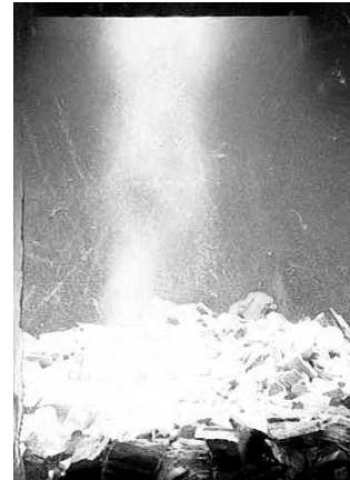
Figure 6: Photo of the smoke vortex during cold experiments in the window reactor.
