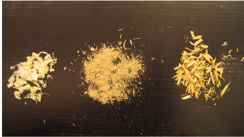
Figure 3 Wood chips from Junckers Industries. a) Softwood shavings b) Beech (hardwood) c) Pinewood (softwood).
