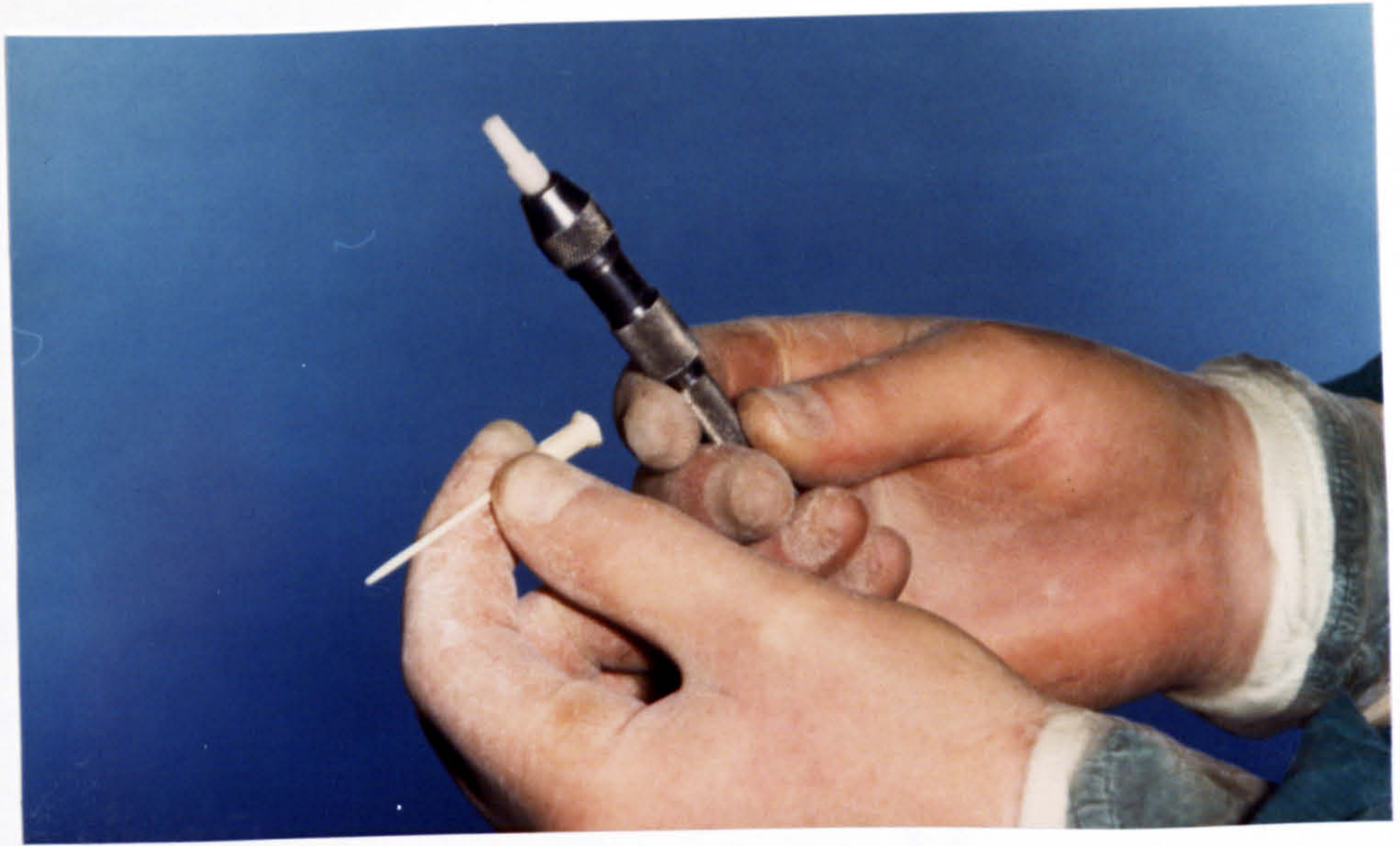
Figure 46 Handpiece-nozzle lure lock assembly
