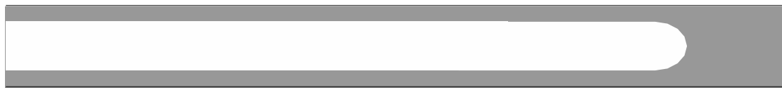
(b) Melt filling stops and gas injection completes filling (primary gas penetration)
