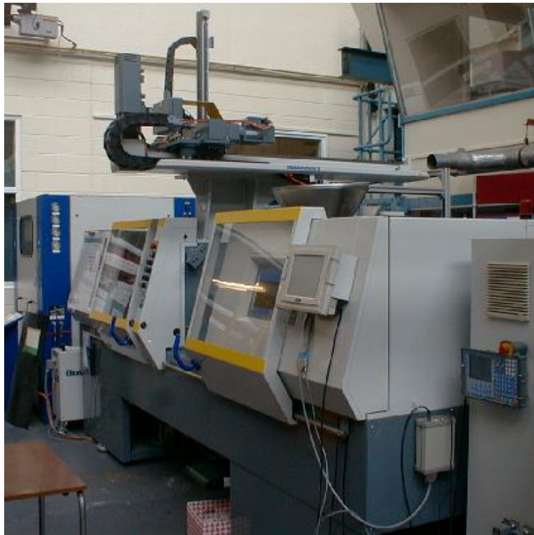
Figure 1.11: The Battenfeld CDK750 with Airmould
