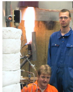
Figure 3. The bright straw gas flame during the first start-up of the 50 kW LT-CFB plant at DTU.
