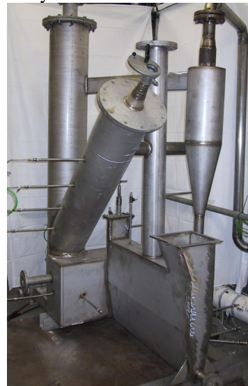
Figure 9: 100 kW Laboratory gasifier (Before insulation)
